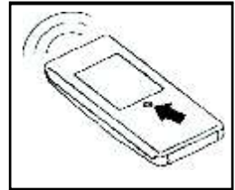
1c. Press "channel-setting" key. The red light will then flash on the motor, you must then press again until it goes off.
